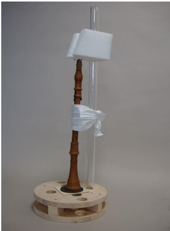
Figure 16: Mounting of a clarinet and oboe on the rotary table
