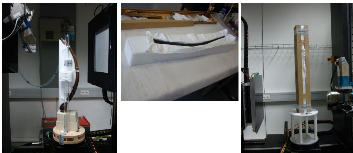
Figure 17: left: English horn with individual supporting foam structure; middle: cornetto in foam block; right: fixed foam block with two cornettos on the rotary table.
