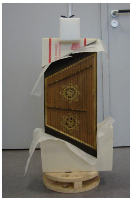
Figure 21 Dulcimer on an individual mold of foam on the wooden base (left); hurdy-gurdy between two base elements, additionally fixed with tape (right)
