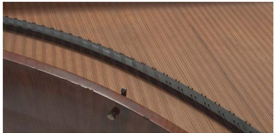
Fig. 7 *The back-pinning in the bridge*
