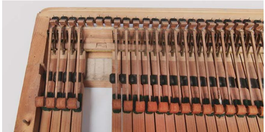
Fig. 11 *The adjustable escapement*
