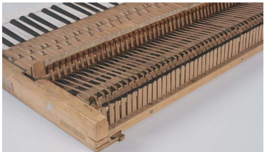
Fig. 10 *Detail of the hammer action seen from behind*
