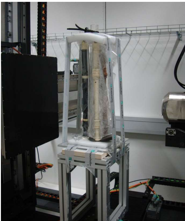
Four 18 th century recorders in a scalable stand and climate-protective wrapping; to the left the X-ray detector, to the right the X-ray source
