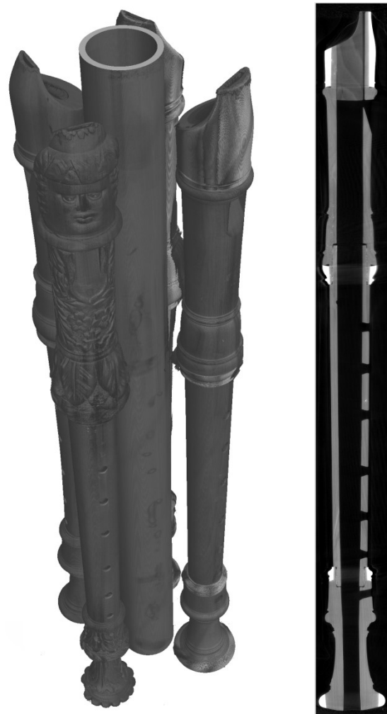
3D-CT view of the cluster of recorders and cross-section of a single instrument
